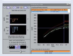
This efficiency vs. flow plot shows a drop in efficiency, for an offshore gas reinjection compressor, indicating deposit build-up on the impeller.
