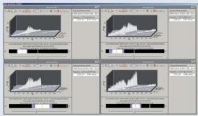
The order based waterfall plot above is useful in identifying unbalance, misalignment and other speed-related faults. Order plots vs. speed below
