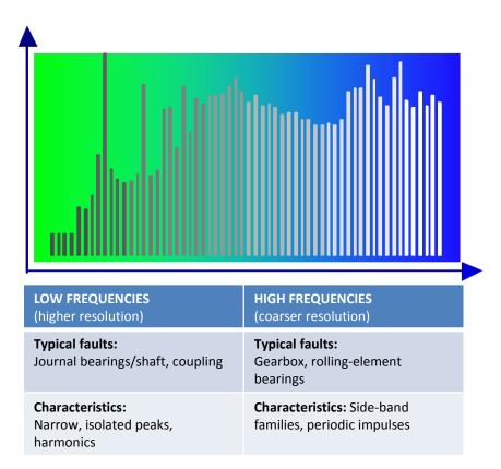
Figure 3. CPB has optimal resolution for detecting many kinds of faults.
