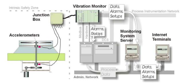
Figure 2. Typical combined safety and predictive monitoring application shown for an air cooler. For some applications a single accelerometer is sufficient for monitoring both bearings. A single accelerometer is sufficient in many cases for monitoring both bearings, if a dedicated monitoring technique is used such as a CPB measurement.
