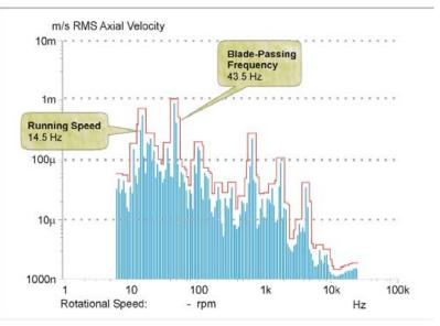
Figure 3. 6% CPB spectrum plots of a cooling fan at a gas processing plant. Lower plot shows a normal signature, upper plot shows resonances excited by a bearing fault.
