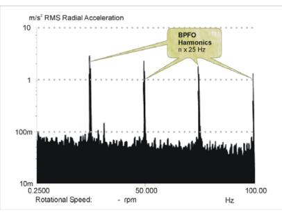
Figure 4. SED spectrum plot showing an outer-race bearing fault.
