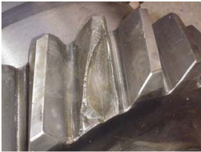
Figure 6. The broken tooth section of the pinion gear.
