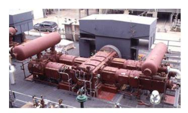
Figure 1. Reciprocating compressors play a significant role in the petrochemical industry.
