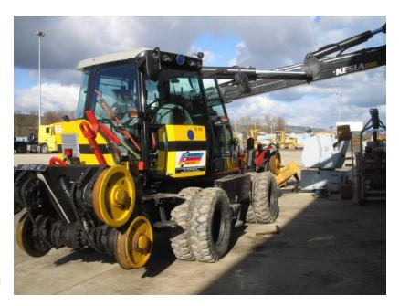
Figure 1. The railroad version of the land clearing tractor .
