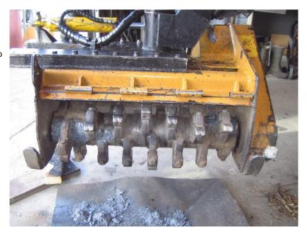
Figure 2. Close-up of the rotary mulcher head of the land clearing tractor, showing the rotor that has to be balanced.
