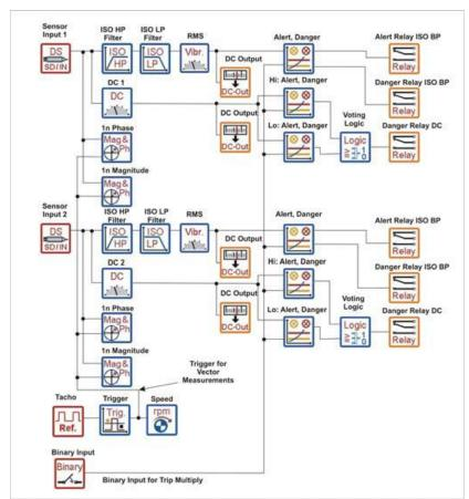
Figure 6. Signal flow diagram for the compact monitor for monitoring the generator and turbine guide bearings.
