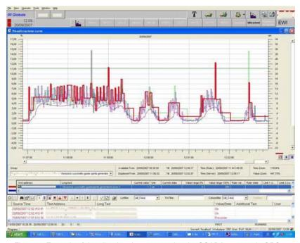
Figure 7. Example of the vibration data exported to the SCADA system via OPC interface. The screen picture above shows vibration data plotted against process parameters such as speed and active power. The Compact monitor has its own remote monitoring software and database (xms), but this is not needed for this application, as this is done by the SCADA system.
