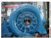
Figure 1. Andritz Hydro workshop in Schio, Italy. (The spiral case and distributor shown in the photo is actually part of several older units that are being reconditioned to be installed in rural South American towns through a non-profit organization. Retired Andritz Hydro factory workers are being asked to come back part time to do the reconditioning and commissioning.)
