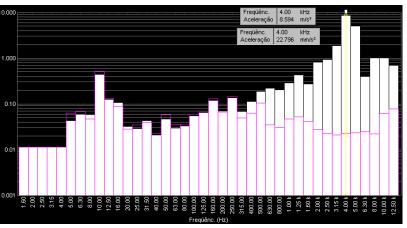
Figure 4. CPB23% of the spiral shaft bearing of the classifier.
