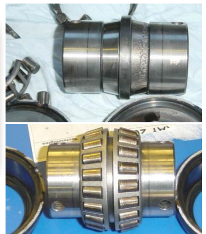
Figure 3. Location (top) and view (right) of the damaged bearing in the centrifugal dryer.
