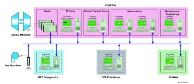
Figure 2. Tele-monitoring system configuration at Copesul and the three participant downstream companies that are using COMPASS.
