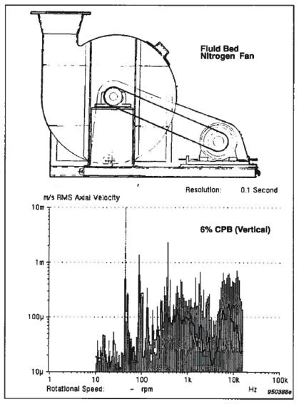
Figure 2. This 75 kW fluid-bed fan from the Melinar factory is used to put a layer of  $N_2$  over the product to increase its resistance to oxidisation. The COMPASS system alerted maintenance personnel to a problem of high frequency vibration on both the horizontal and vertical CPB readings from measurement points located on one of the fan's bear ings. Attributed to a bearing defect, an inspection found fretting corrosion on the outer race.
