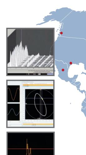
Examples of the powerful plotting functionality of **Compass 6000™**. Top to bottom: Waterfall spectrum plot, orbit plot, multi-trend plot
